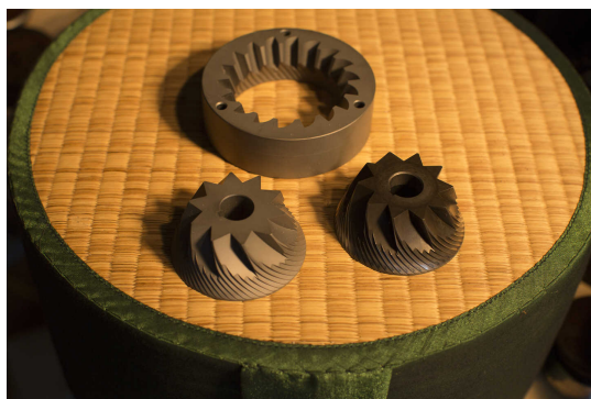
Figure 4. Conical burrs out of a grinder
