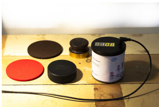
Figure 21. Tonino roast color meter, hardware and software (open source) by Marko Luther
